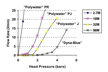
Very low pressure (< 4 psi or 0.25 bars) would pump the 2,700 cps liquid Polywater® PR at adequate flow rates. The highest viscosity lubricant, Dyna-Blue® (98,000 cps) required 60 psi or 4 bars to flow at satisfactory rate. The outlet hose was 20 feet (6 m) in length with a 0.75 inch (19 mm) ID in this test.
