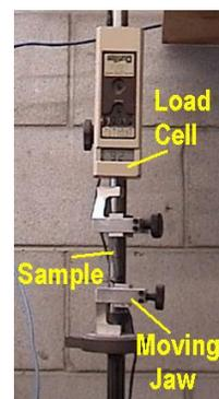
For the adhesive shear test, the strip is clamped into a pulling device and pulled apart at a rate of two inches per minute. Pulling force readings are the maximum force before breaking. The value shown is the average of three pulls. These values may vary with application technique, field conditions and the actual material.
