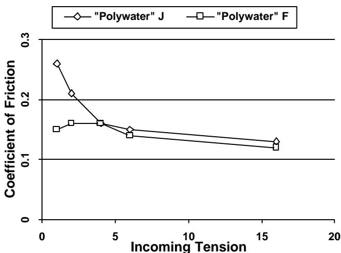
To explain the graph, first you must know that Polywater® J and Polywater® F are two of American Polywater's high-performance cable pulling lubricants ("J" is usually used for electrical cable and "F" for fiber optic cable). They are similar chemically, except that "J" is a gel lubricant (higher viscosity) and "F" is a liquid.
