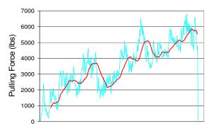
Graph 1. Polywater<sup>®</sup> J Tensions vs Pulling Time
