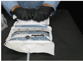
Burst primary seal
