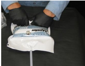
Burst secondary seal
