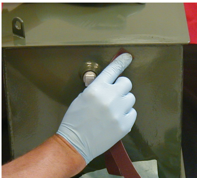
Sand or brush repair area
