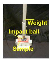
approximately <sup>1</sup>/<sub>8</sub>-inch thick. The patch is allowed to cure and harden for 1 week. The coated substrate is clamped into an attached base that positions the cured adhesive exactly center to the falling weight. Impact resistance is determined as the amount of energy required to cause a crack in the adhesive seal.
